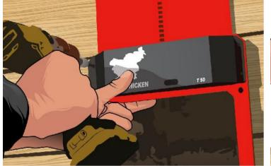
**!MANDATORY PROCEDURE!** Unscrew the 4 screws on the black drive unit.
