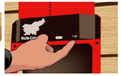
Press the test switch to see if the device is up and running.
