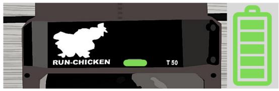
GREEN LIGHT - Blinking means that the battery is full and that the unit is active// UP AND RUNNING.
