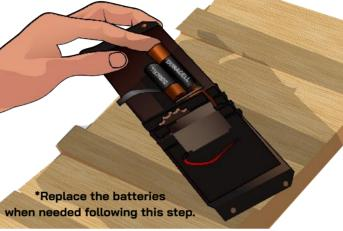
drive Remove the unit and check/place batteries inside.
