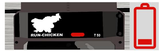
**RED LIGHT**- Blinking means that the battery is empty or almost empty. In this case you need to replace the battery. approx. 20 days prior fully empty batteries.
